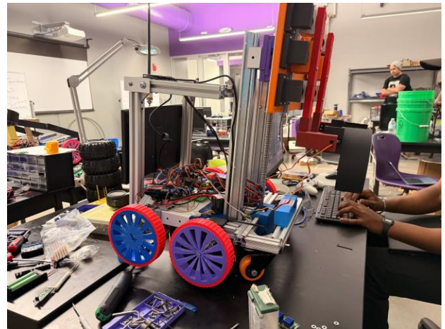
Fig. 8. WonkyBot fully assembled — side view, April 2026. Belt-drive transmission, aluminum extrusion chassis, and wiring visible.
